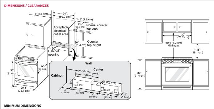
\*30" (76.2 cm) minimum clearance between the top of the cooking surface and the bottom of an unprotected wood or metal cabinet; or 24" (60.9 cm) minimum when bottom of wood or metal cabinet is protected by not less than 1/4" (6.4 cm) flame retardant millboard covered with not less than no. 28 MSG sheet steel, 0.015" (0.381 mm) stainless steel, 0.024" (0.610 mm) aluminum or 0.020" (0.508 mm) copper.
